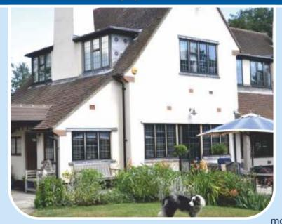
At just 33mm front to back, our Royale Steel Replacement Windows are one of the slimmest thermally broken aluminium window systems on the market. With slim profiles replacing steel windows has never been easier - with no cutting back of plaster, brick or wooden sub-frames, speeding up installation times and reducing costs.
